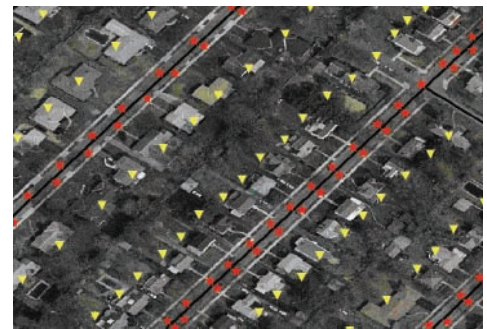
MapMarker ParcelPrecision offers both centroid locations (yellow triangles) and interpolated street offset locations (red stars).
